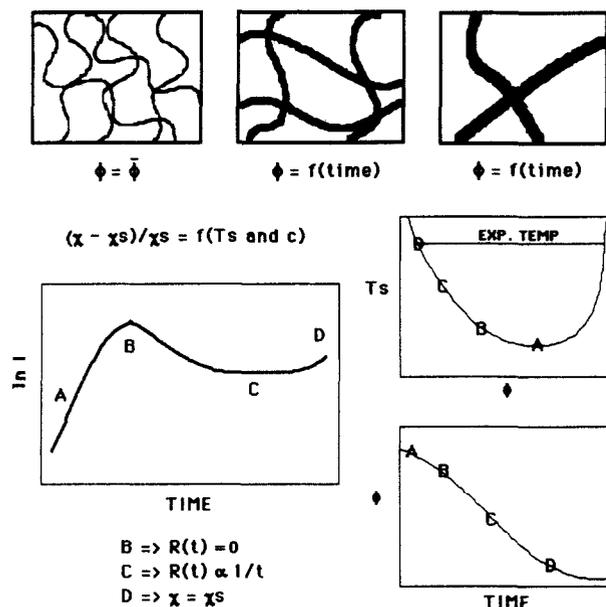
**Figure 11.** Self-similarity in intermediate stages on polymer phase separation. (Dark lines in the top figures indicate, schematically, regions of composition fluctuations. Magnification remains constant in the top three figures.)
