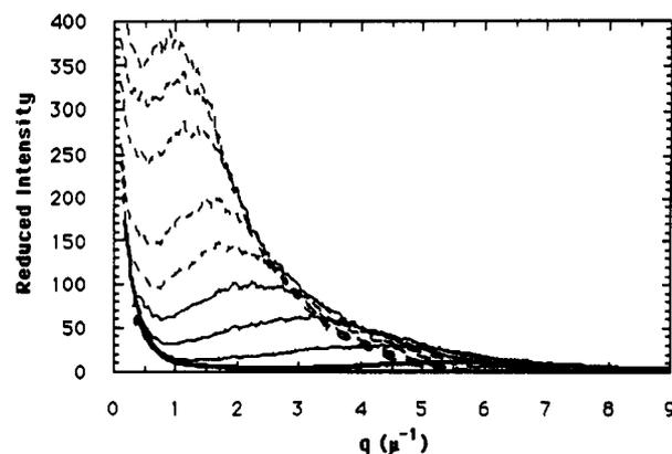
**Figure 3.** Series of light scattering measurements for atactic PVME blended with PS (75% PVME) at 123 °C. (The critical temperature is 121 °C.) The patterns are separated by about 1 min and monotonically increase in intensity with time.
