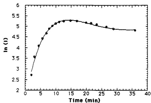
**Figure 12.** Typical fit of the scattering data using the pseudospinodal approach and the F-H-S equation for  $(g - g_s)/g_s$  (eq 5.24). (123.5 °C, heterotactic PVME/PS,  $q = 1.84 \mu\text{m}^{-1}$ .)
