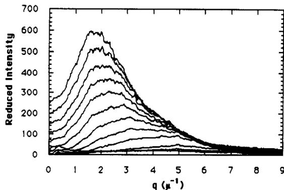
**Figure 2.** Series of light scattering measurements for isotactic PVME blended with PS (75% PVME) at 130 °C. (The critical temperature is 109 °C.) The patterns are separated by about 1 min and monotonically increase in intensity with time.
