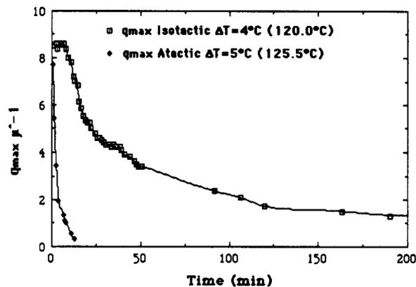
**Figure 4.**  $q_{\text{max}}$  versus time for isotactic and atactic PVME/PS blends of about 4 °C quench.
