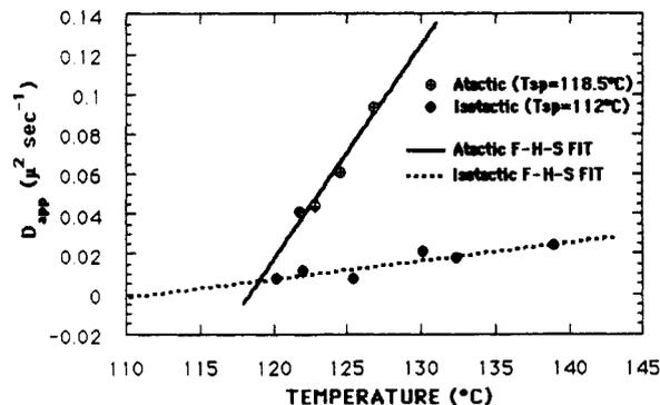
Figure 9.  $D_{app}$  versus quench temperature for 75 wt % isotactic and heterotactic PVME/PS blends for extrapolation to the spinodal point at  $D_{app} = 0$ . Lines are F-H-S fits using  $(-K_c T)(g - g_s)/g_s$  (with  $K_c$  as the only fit parameter) for the isotactic and atactic blends.
