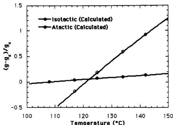
Figure 1. Predicted behavior for  $(g - g_s)/g_s$  from the F-H-S analysis. This is the thermodynamic driving force for phase separation above the coexistence curve. Isotactic PVME shows lower miscibility and much slower kinetics above the miscibility limit  $(g - g_s)/g_s = 0$ .
